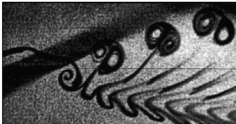
Figure 14. Streak lines, experimental data by Jones and Platzer - Sr = 1.5
