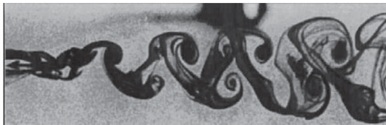
Figure 5. Streak lines, experimental data by Jones and Platzer - Sr = 0.29
