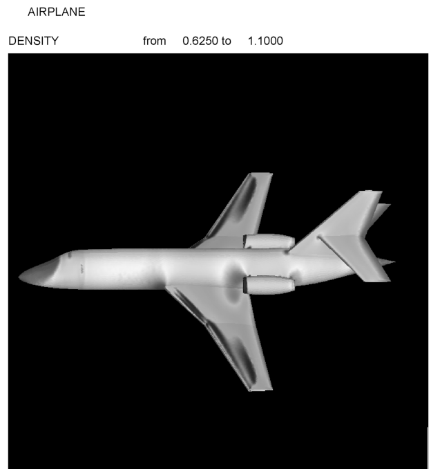
Fig. 17 Density contours for a business jet at M = 0.8 , \alpha = 2 .
