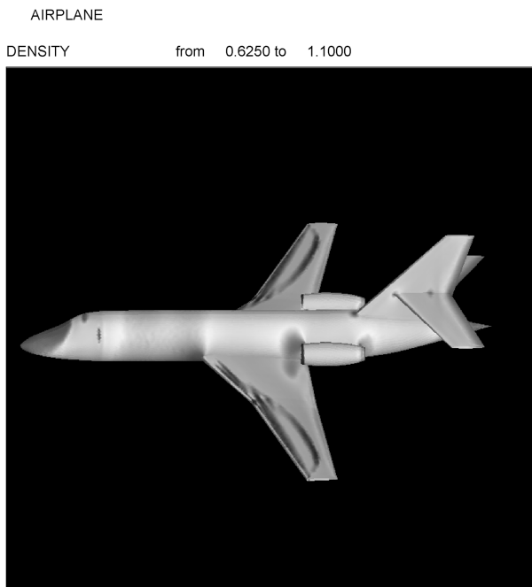
Fig. 21 Density contours for a business jet at M = 0.8 , \alpha = 2.3 , after redesign.
