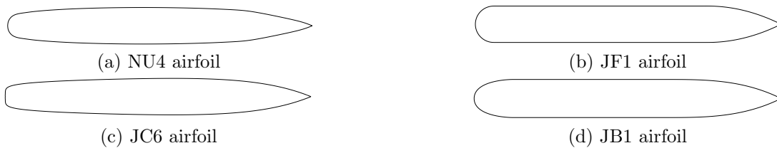
Figure 1. Geometric shapes of a set of 4 symmetric airfoils admitting non-unique transonic solutions.
