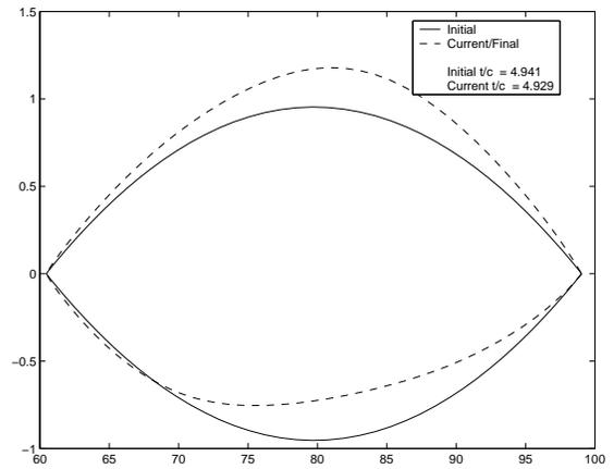
Figure 2: Sonic Boom Minimization: Initial and Final Airfoil Shape After 50 Design Cycles.
