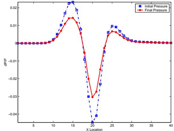
Figure 3: Sonic Boom Minimization: Target, Initial, and Final Near Field Pressure Distribution After 50 Design Cycles. Mach = 1.5,  $\alpha = 1.75$  deg, Fixed Lift Coefficient = 0.05, Fixed Thickness Ratio
