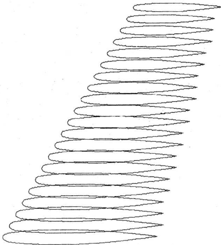
FIGURE 4. GEOMETRY OF ONERA WING.
