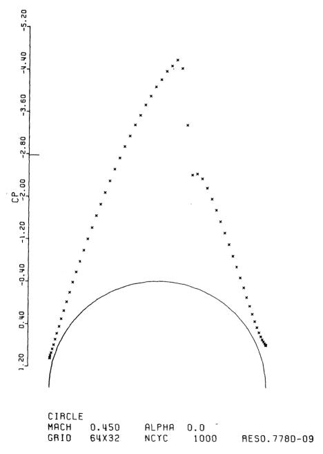
Figure 2a. Pressure Distribution of Transonic Flow Past a Circular Cylinder
