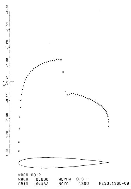
Figure 3b. Euler Solution for Transonic Flow Past an NACA 0012 Airfoil
