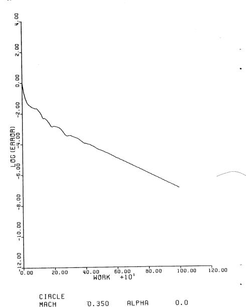
Figure 1b. Convergence History for Subsonic Flow Past a Circular Cylinder
