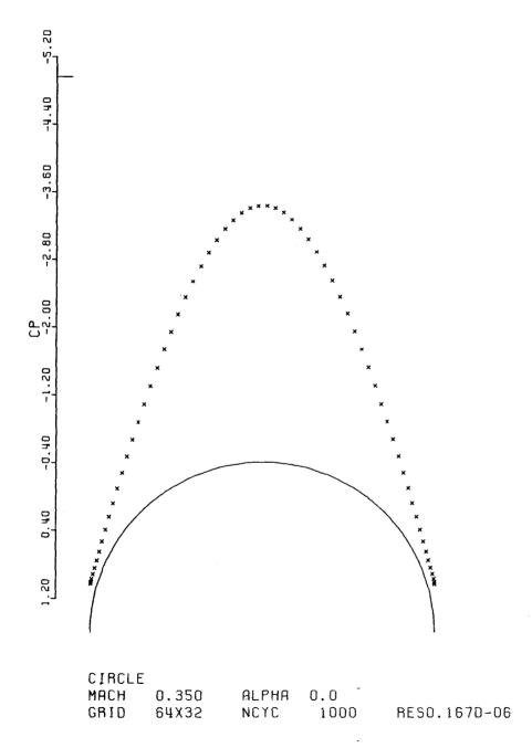
Figure la. Pressure Distribution of Subsonic Flow Past a Circular Cylinder
