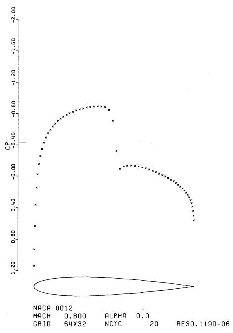
Figure 3a. Potential Flow Solution for Transonic Flow Past an NACA 0012 Airfoil
