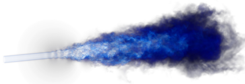
Fig. 11. Instantaneous velocity magnitude field of the incompressible jet at t = 1500 .
