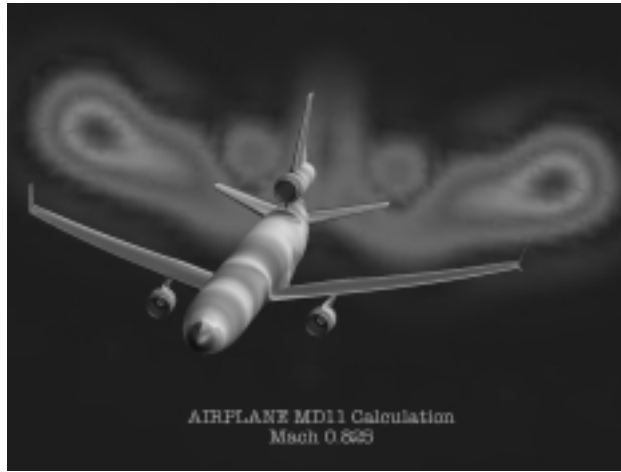
Figure 12: Computed Pressure Field for a McDonnell Douglas MD11
