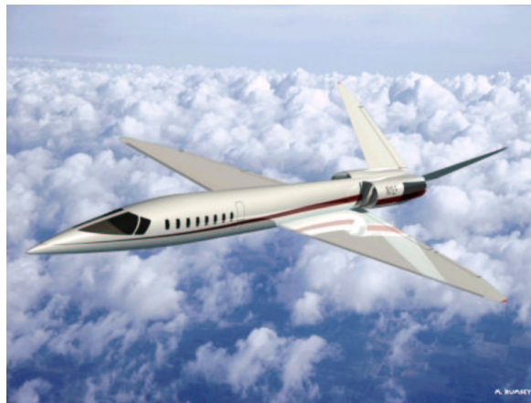
Fig. 2 Natural laminar flow supersonic business jet configuration.
