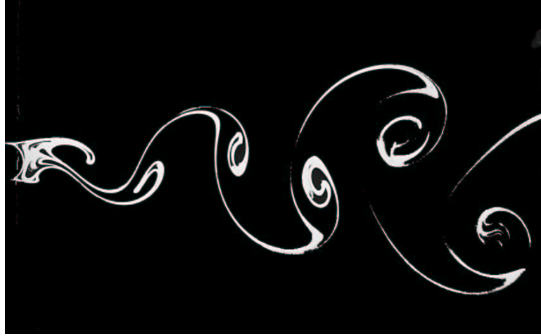
Figure 3.1: Smoke visualization of laminar vortex shedding in the wake of a cylinder at a Reynolds number of 140. Experiment conducted by Taneda [63] and reproduced by Van Dyke [17].
